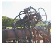
A complex network of hydraulic valves and hoses direct fluid to either the front-mounted loader and bucket, or to the rear-mounted 3-pt. hitch.
