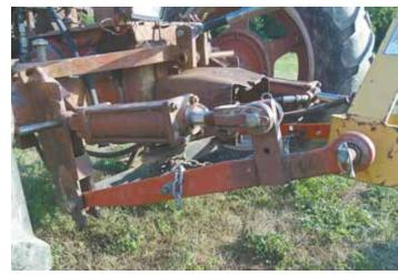
He used 3-in. bore and 16-in. stroke cylinders for the lift arms and as an option for replacing the top-link arm.
