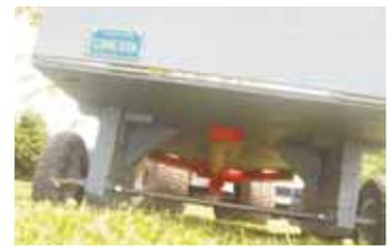
Trailer rides on four 10-in. wheels mounted on 5/8-in. threaded rod axles fixed to wood brackets. Axles move up and down inside oblong slots in wheel mounts.
