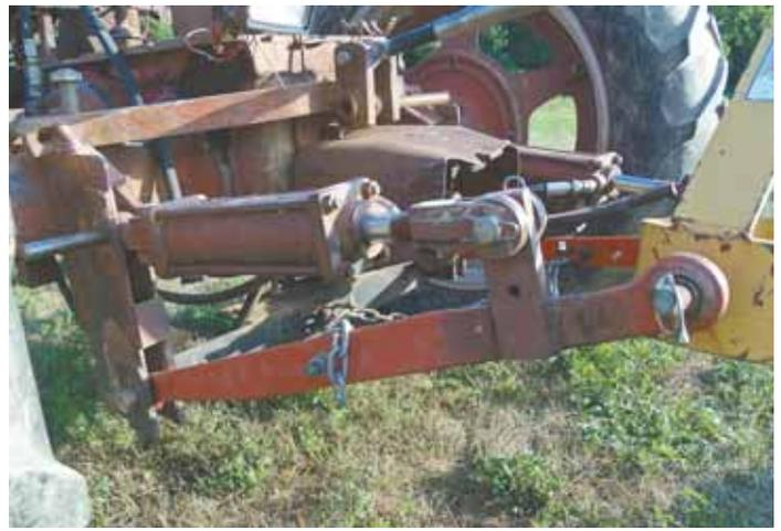
He used 3-in. bore and 16-in. stroke cylinders for the lift arms and as an option for replacing the top-link arm.
