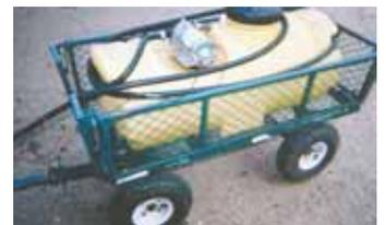
**Carlson removed the nozzle from a spot spray wand and tows a tank behind his lawn tractor. When he squeezes the trigger, the pump kicks in.**
