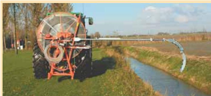
**Power Jetter works like a giant snake to unplug drainage tile without digging it up. It slowly pushes a solid plastic hose into tile line while injecting a stream of water at up to 500 psi.**
