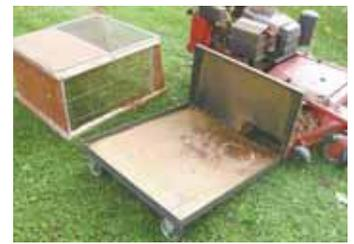
Leaf catcher pins onto side of walk-behind mower and has a plywood frame that rides on two caster wheels. A 3-sided "catcher box" friction fits into the angle iron frame.
