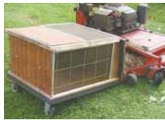
Leaf catcher pins onto side of walk-behind mower and has a plywood frame that rides on two caster wheels. A 3-sided "catcher box" friction fits into the angle iron frame.
