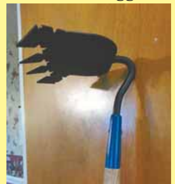
Pronged garden hoe's blade is equipped with a series of 2-in. prongs.
