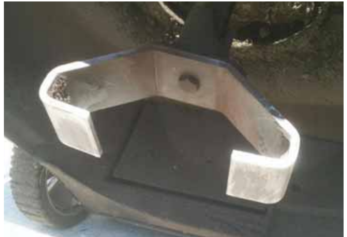
"Tiger Tiller" is a 10-in. wide curved steel tiller blade that bolts onto the original blade mount on a riding mower. It's designed to loosen dirt in small areas.
