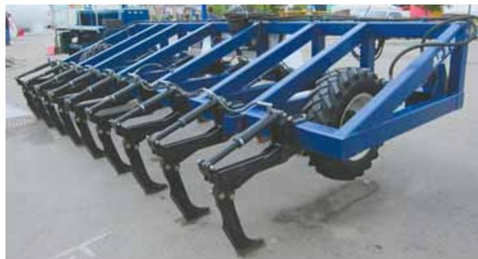
AgrowPLOW shanks are spaced 26 in. apart on each of 2 toolbars. Shanks are staggered, which results in only 13-in. spacing between shanks for better fracturing action.
