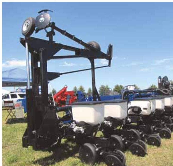
A-M-E Co. planters use an open design construction that allows use of off-the-shelf attachments and accessories. “You can get your planter set up exactly how you want,” says company rep Jim Harken.
