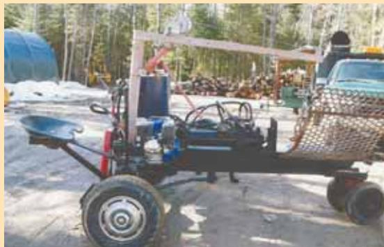
Wayne Langlois's wood splitter is fitted with a crane with tongs. It lifts heavy chunks onto a metal pan and then up onto the splitter table.
