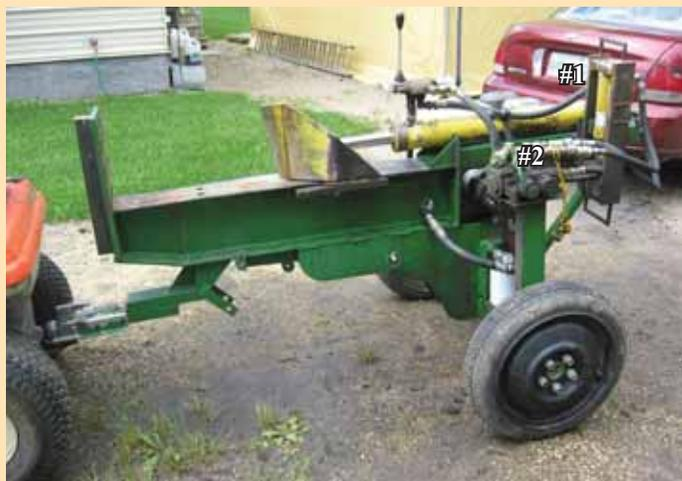
Ross St. John's home-built wood splitter is fitted with a hydraulic press (1) and a double spool valve (2) that provides a pair of extra hydraulic outlets.
