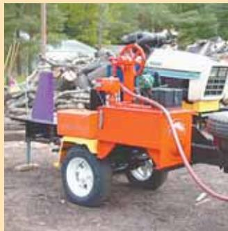
Cub Cadet's engine shaft-drives a hydraulic pump that operates the splitting cylinder. The Cub's battery and alternator were replaced with a 100-amp car battery and alternator. Return oil from the hydraulic pump goes to a hydraulic motor that belt-drives the alternator.
