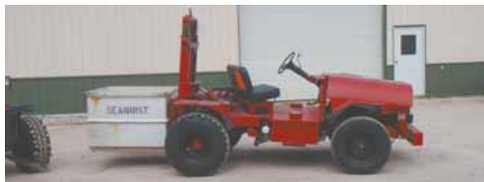
Dale Seaquist custom-builds forklifts for orchard use by modifying 3/4-ton, 4-WD pickups with special lift forks and an air bag suspension system.
