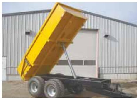
Berkelmans trailers are custom-built with heavy-duty hydraulic hoists and powered tailgates. "Dump trailers are a lot cheaper to own and use than dump trucks," says Bill Berkelmans.
