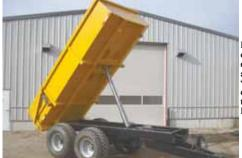
Berkelmans trailers are custom-built with heavyduty hydraulic hoists and powered tailgates. "Dump trailers are a lot cheaper to own and use than dump trucks," says Bill Berkelmans.
