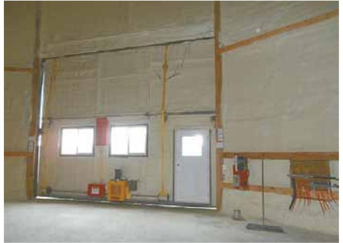
Measuring 16 ft. high and 20 ft. wide, bifold door is complete with windows and a walk door.
