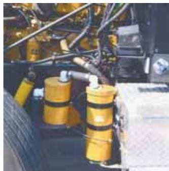
George Muth keeps engines clean by using two aluminum canisters and a hose that runs from the breather tube outlet at the valve cover.
