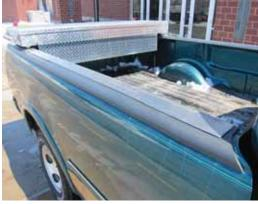
Toolbox travels on 2 aluminum rails that clamp to top of pickup bed. Four wheel bearing rollers are mounted under toolbox.
