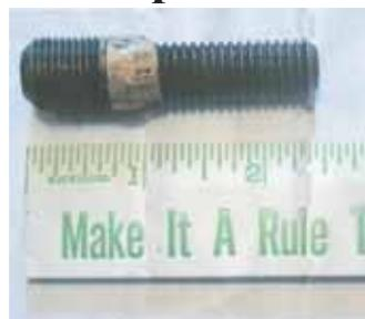
**To make adapter Rice cut the threaded end off two different size bolts, then brazed the cut ends together and bored a hole through entire assembly.**
