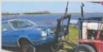
"A pipe across the bottom with steel hooks on it attaches to the vehicle's frame. Vertical strips of 1-ft. wide, 3-ft. long baler belting form the sides, with more belting and chain hooks on top."
