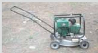
**Robert Boddy, Bloomingfield, N.Y.:** "I mounted an electric generator to the base of a push lawn mower. It makes moving the generator from place to place much easier. Real handy."
