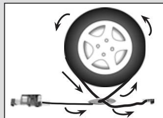
around the tire and through a heavy-duty washer. Hook both ends of the come-along in opposite directions and in line with the centerline of the tire. When it goes through the washer this way it'll form an X.
