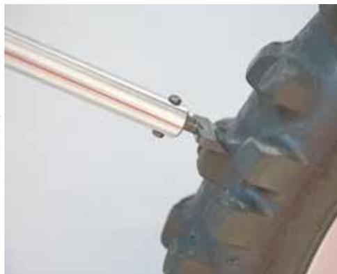
Heated, carbide cutting blade slices away rounded edges on worn tire treads to boost traction.
