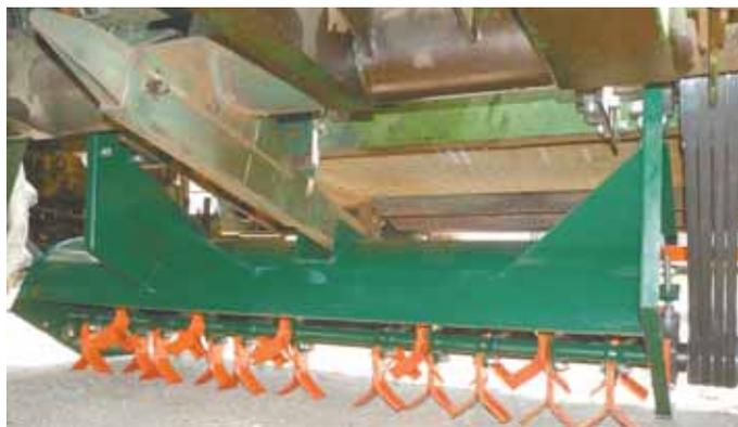
Chop Rite stalk chopper mounts under New Idea pull-type corn pickers and is belt-driven off the picker gearbox.
