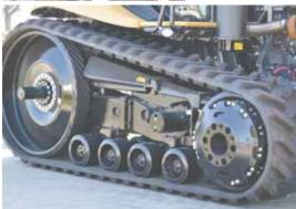
Worn-out rubber on bogie wheels can be replaced with cast urethane, which will make the wheel last longer and costs half as much as buying a new one, savs Green Rubber-Kennedy Ag.
