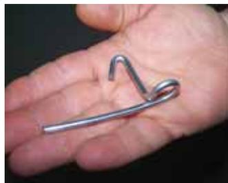
T-post “staple” is made from high-tensile galvanized wire and forms a loop in the middle.
