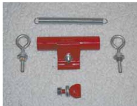
Kit resolves the net wrap malfunction on Case IH and New Holland balers, providing even tension on the brake arm that stops and cuts the wrap.
