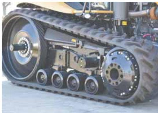
Worn-out rubber on bogie wheels can be replaced with cast urethane, which will make the wheel last longer and costs half as much as buying a new one, says Green Rubber-Kennedy Ag.
