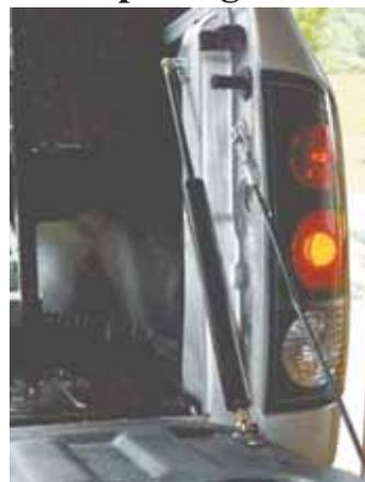
Lift assist kit uses a gas spring to slowly lower pickup tailgate and close it effortlessly.
