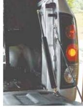
Lift assist kit uses a gas spring to slowly lower pickup tailgate and close it effort-lessly.
