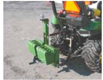
Parnow’s 3-pt. mounted “Heavy Hitch” accepts up to 600 lbs. of suitcase weights and comes with a wheeled storage cart. Weight frame includes a standard 2-in. receiver hitch. An optional second receiver hitch can be installed top-center on the frame for moving gooseneck trailers.
