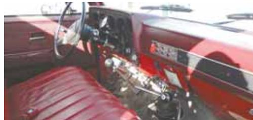
Closed center system uses solenoid-operated, hydraulic valves. To control the hydraulics, Ray installed a mechanically linked 8-ball shifter in the cab for the pto.
