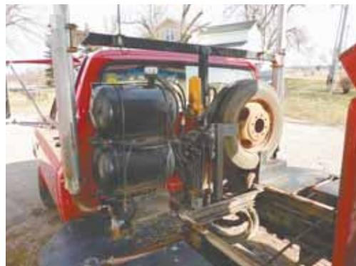
He stripped off the old bed and built a shorter 10-ft. bed. That left room for an 18-in. sub bed behind the cab to mount hydraulic reservoir tanks, a spare tire and exhaust stacks.
