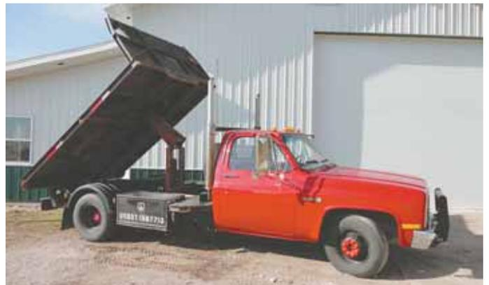
Ray Lee converted a conventional bed 1982 GM 3500 pickup into this lift bed model that's also equipped with hydraulics and a winch.
