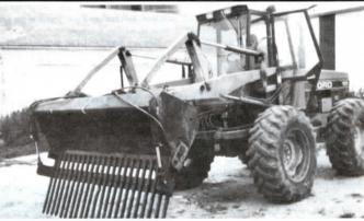
This "stone fork" mounts on the front edge of an 8-ft, loader bucket and pivots up or down, powered by a pair of hydraulic cylinders. When scooping up rocks, I hold the bucket close to the ground, tilting the front of the bucket up and the 3-ft. long forks down so they just skim the surface. Rocks roll up onto the forks, then slide down into the bucket.
