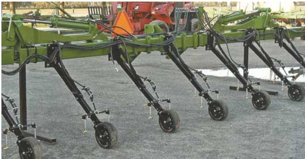
Photo shows a 12-row layby rig on 38-in. rows set up with Estes’s aftermarket kit. It lets you spray herbicides beneath the crop canopy using your existing toolbar.
