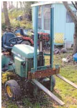
Forklift mounts on a snowplow mounting bracket on Gorge’s Deere garden tractor. Forks are attached to a carriage that’s raised up or down by a hydraulic cylinder.
