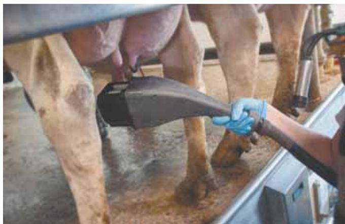
Hand-held brush uses a chlorine dioxide cleaning solution to wash, disinfect, stimulate and dry teats in one easy step.
