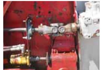
Because of the angle of the framework, they had to put a double yoke on the beater driveshaft before it enters the gearbox.
