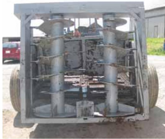
The Bowmans jobbed out the construction of the beaters to an auger specialist. Flighting on the 36-in. dia. beater was made from 3/8-in. steel.
