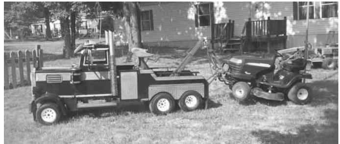
Stockton's 9-ft. wrecker has air intakes on the sides and a forward tipping hood. The metal cab and body were fashioned from a 300-gal. fuel tank.
