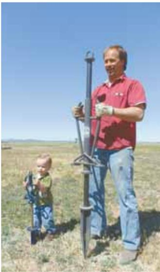
All-Tie Anchor Post has a 4-bladed spear point with a sliding pounder on the post that's used both to pound in posts and pull them out.
