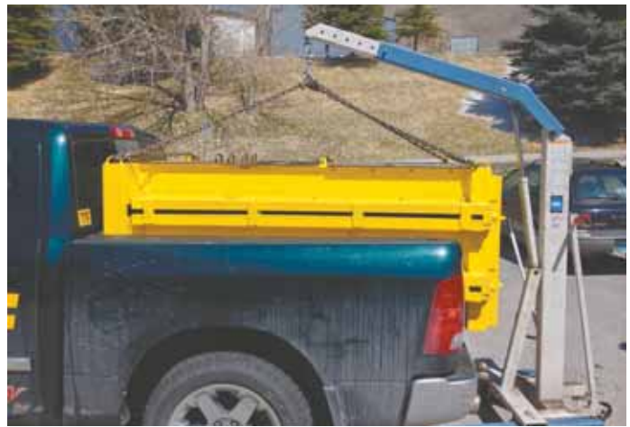
Battery-powered BioPac'r compactor is loaded by hoist into pickup bed.
