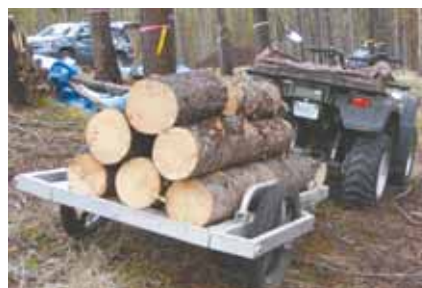
When empty, Backpacker Cart rides on the rear rack of an ATV. To use it, you just fold it out and hook it up to the ATV. Works great for hauling logs, etc.
