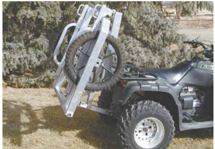
When empty, Backpacker Cart rides on the rear rack of an ATV. To use it, you just fold it out and hook it up to the ATV. Works great for hauling logs, etc.
