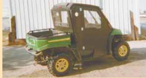
Roy Viel built a new cab for his Gator 550 utility vehicle for less than \$500. All cab panels bolt to existing holes in the vehicle's roll cage.
