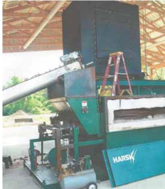
Marsh Farms' poultry litter gasification system can produce up to 30 kilowatts of electrical power annually. Clean, hot air is used to heat the poultry barns.
