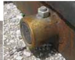
To mount bale spears, Schweppe pushes spears through welded-on bushings and out the back, then inserts a 1/2-in. bolt through holes already in each bushing.
