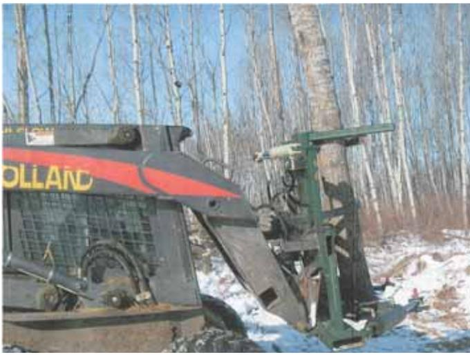
Skid loader-mounted tree shear has stationary, V-shaped guide arms on top with a pair of curved metal grapple arms below them. Cutting blades are at bottom.
