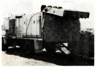
rig for compacting loose hay into large rectangular bales, or for compacting regular hay bales to half their size to increase the payload for shipping. His labor-intensive operation, using bundled hay pitched in by hand, turns out one big bale every 20 minutes, with half of
