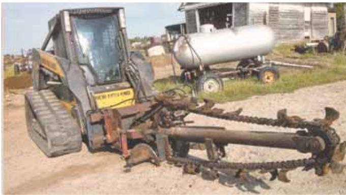
"It does the work of much more expensive machines," says Chuck Hardenburger, who converted an old 3-pt. trencher into a skid loader-mounted model.
