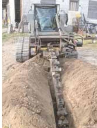
He bought a used hydraulic motor and attached it to the trencher's chain-drive system.
