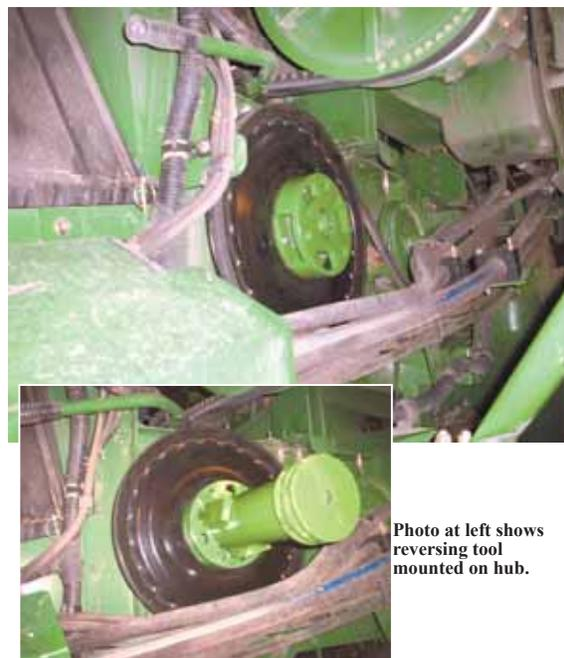
**Special hub fits over the pulley of combine's discharge beater, allowing you to use Deere's reversing tool to clean out a plugged beater.**
