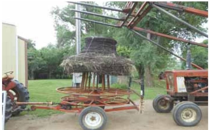
**Once the reel is full, a loader tractor is used to lift the big spool of wire off.**
