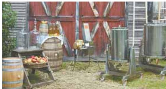
Lanman water press uses a flexible rubber bladder to produce as much as 3 gal. of cider from a bushel of apples.
