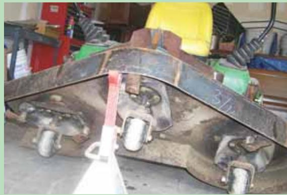
Front-mount mower deck is designed with the caster wheels underneath the deck – rather than out front – and new-style mower blades that rotate around them.
