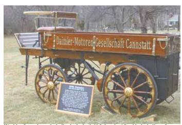
Working from photos, he built a body that's 11 ft. long by 4 ft. wide, including a footrest for the operator.
