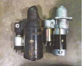
Gear reduction starter provides the extra cranking speed needed to turn over a tractor's engine without running down the battery Photo shows stock starter at left.
