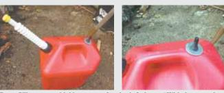
Brent Gill came up with his own vent for plastic fuel cans. "With the core valve removed, it's easy to fill a tank because air rushes in through the valve when the cap is removed," he says.
