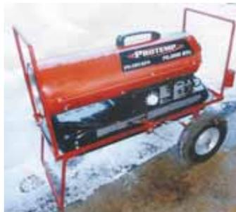
as a base to stand on. I didn't want to drag it around or let it set on the concrete floor, so I decided to use some shop scrap and a pair of wheels to make a rolling base for the heater. Makes it easy to move around just where you need it without damaging the tank."
