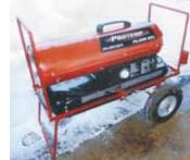
as a base to stand on. I didn't want to drag it around or let it set on the concrete floor, so I decided to use some shop scrap and a pair of wheels to make a rolling base for the heater. Makes it easy to move around just where you need it without damaging the tank."
