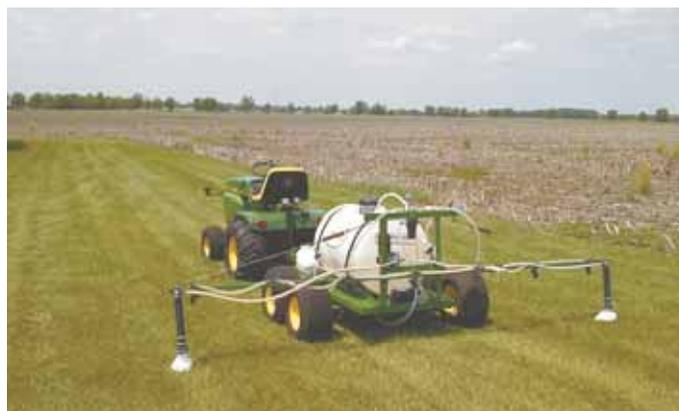
Lyndon Miller's home-built sprayer rides on walking tandem axles and has a folding 10-ft. boom built in sections, as well as a foam marker system to avoid overlaps.
