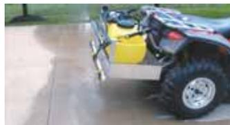
Dennis Brooks mounted a 15-gal. Demco poly tank on an aluminum frame, which slips into the receiver hitch on back of his 4-wheeler.
