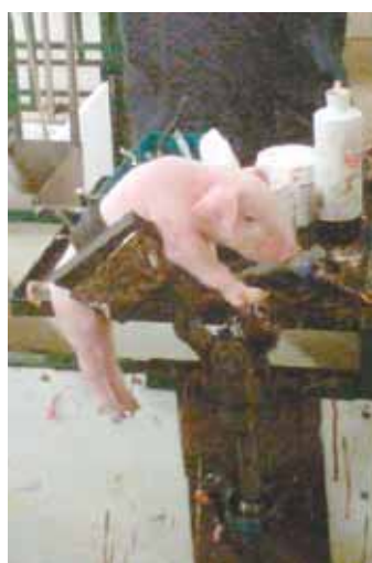
Piglet processing arm is designed to hold young pigs safely while workers do tasks. A universal joint allows arm to be easily turned for access to piglet's head and tail.
