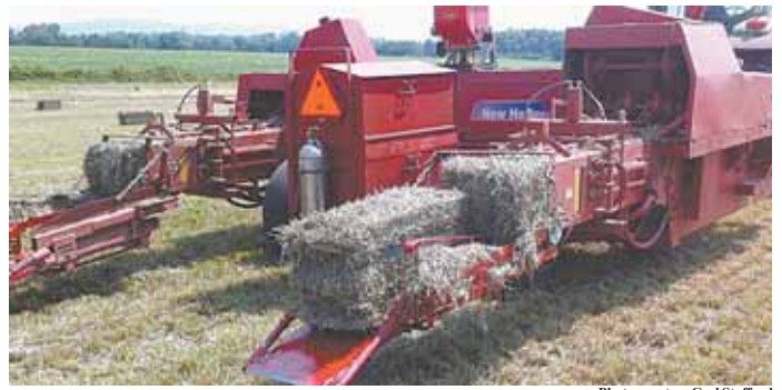
Photo courtesy: Carl Stafford Double baler picks up hay from large merged windrows, separates the inflow into 2 separate chambers, and kicks bales out 2 separate chutes at the same time.
