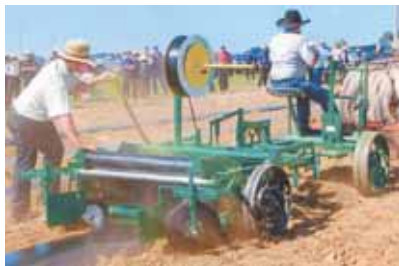
E-Z Trail makes this Hogback raised bed mulch layer, shown here pulled with a forecart behind a team of horses.
