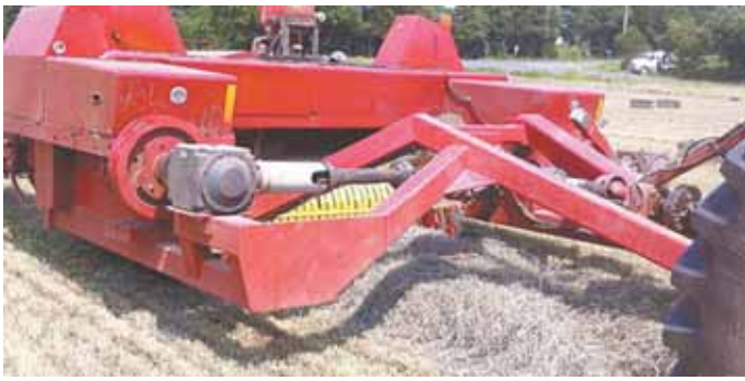
Rusty Inskeep cut up 2 New Holland 5070 balers and combined them into a single machine. "It lets us make more than 900 bales an hour in heavy, first crop hay," he says.
