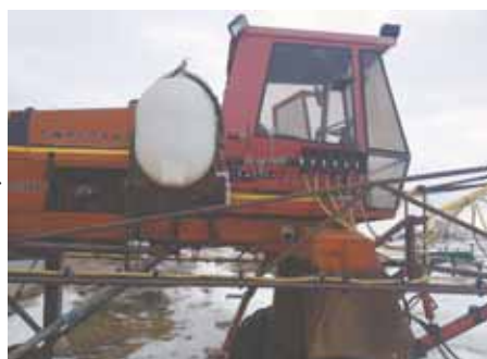
With electric-over-hydraulic valves, the operator can shut off individual booms.
