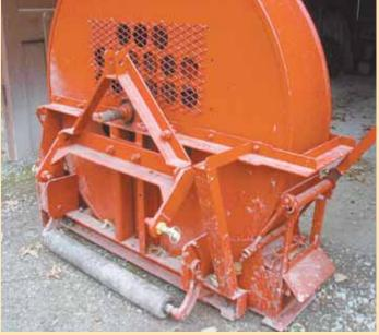
Kurt Cook converted a silage blower into this heavy-duty leaf blower, equipping it with rollers off an old set of reel mowers on front and back so it rolls over uneven ground.
