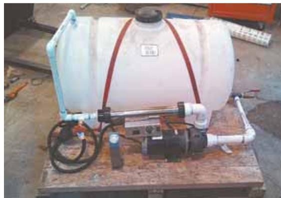
Kerry Kligora used parts from an old hot tub, along with a 65-gal. poly tank, to make a non-pressurized water heater for his gas pressure washer.
