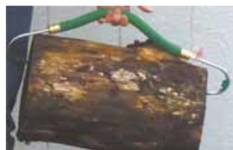
Valley catalog (ph 800 871-8158; www.leevalley.com). My only regret is that I didn't order 2. The sharp hooks on either end of the flexible rubber hose bite into the ends of a chunk of log, while the rubber hose is easy on the hands. It's sturdy and well made. Best of all, it makes it easier to carry larger chunks of firewood to the splitting pile."
