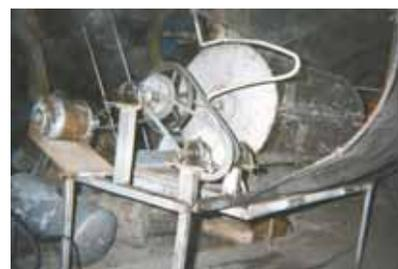
A 1/4 hp. motor belt-drives paddle assembly inside sheller drum.
