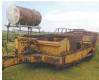
A typical Reynolds scraper before refurbishing, with rusty, bent and broken parts (left) and a typical rebuilt and repainted scraper.
