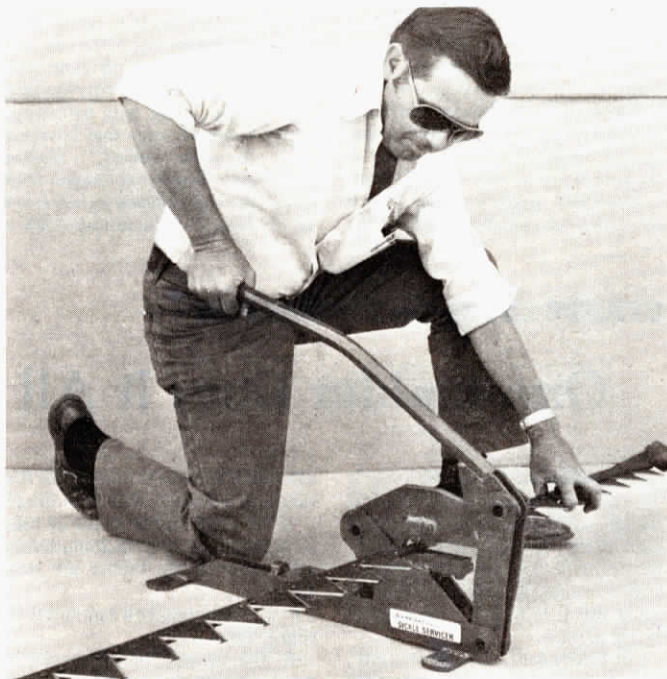
Johnson Sickle Servicer removes and replaces sickle sections for all mower, windrower and combine sickle bars. It will remove old sections, punch out old rivets, and rivet in new sections.
