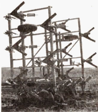
Note the 20 in. coulters in front of each shank for cutting through heavy trash.
