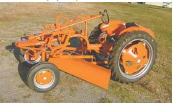
One of Kimball's G's is set up like a mini road grader, and has a home-built blade that hangs on the original turnbuckle/tool lift bar.
